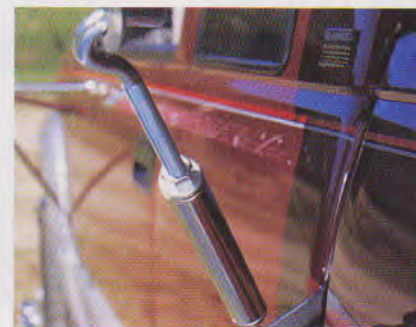
Happijac® chrome-plated anchors are recommended to attach the camper to the truck. The front anchors are spring-loaded to absorb unexpected bounces and are designed to attach to the front of the truck bed with special plates. Rear tie down attaches at the bumper. They're proven to be the safest and strongest camper tie downs and turnbuckles on the market.
