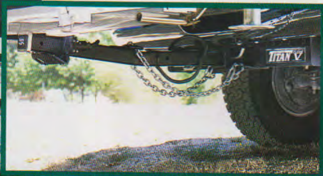
TITAN Class V Receiver with 2 -1/2" tube steel extension bar.
